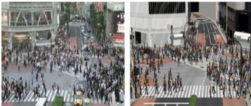
Fig. 9. Comparison between the actual scene (right) and the simulated scene (left) of Shibuya Crossing in Japan. The proposed least-energy model by Guy et al. [104] is able to reproduce the emergent behavior in actual crowd scenes, such as arching and self-organization into lanes, by applying simple and intuitive formulation of rules and biomechanical measurements to the individuals agents and their interactions.
