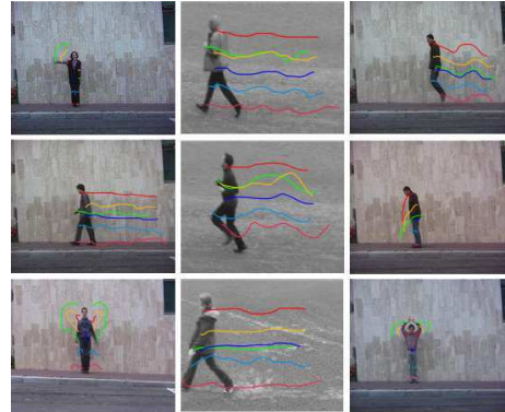
Fig. 1. Sample activities used from the database provided by [1], [16]. Trajectories from seven landmarks (left/right shoulders, left/right elbows, left/right knees and hip) on the human body are quantised and input to our method.
